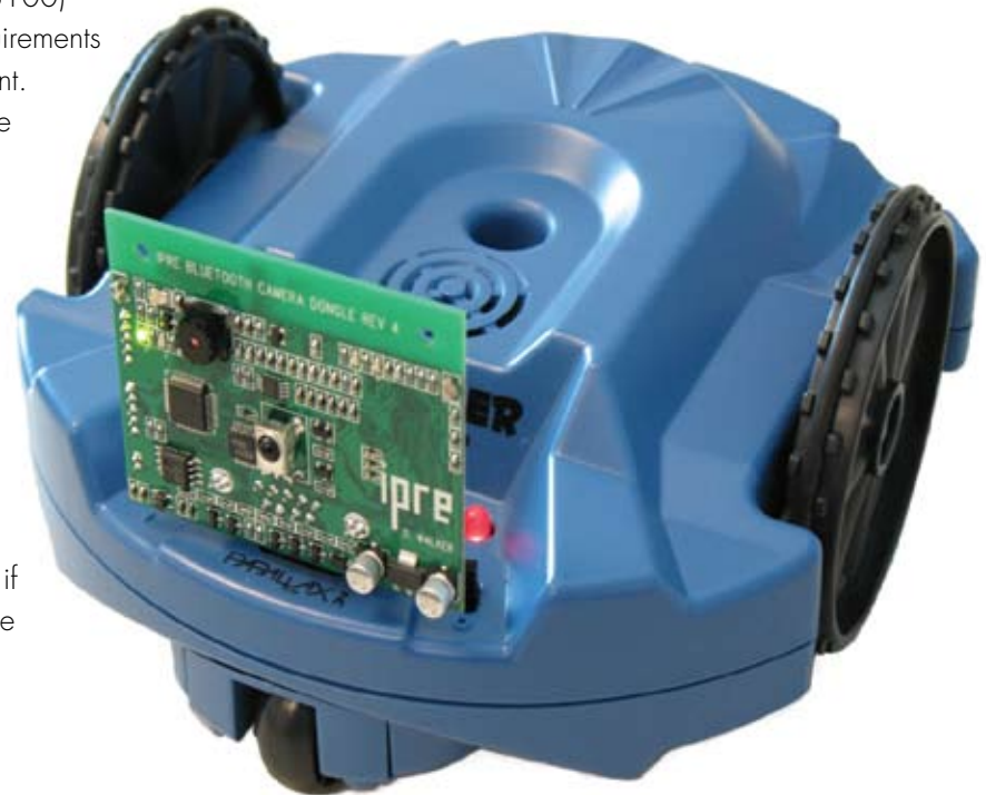
ROBOT UPGRADE MODULE INSTALLED ON A PARALLAX SCRIBBLER ROBOT
