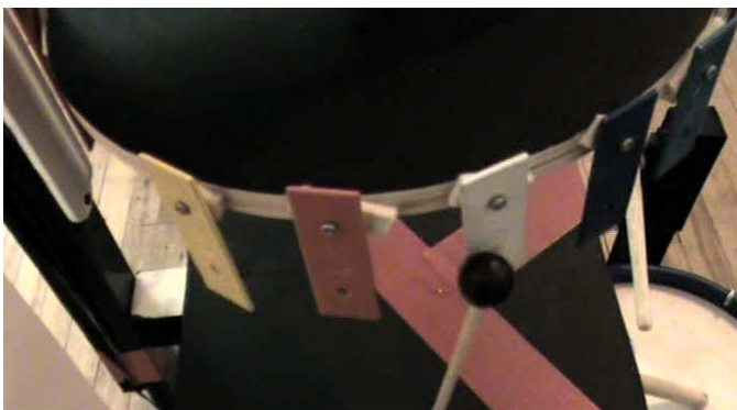
Fig. 3. Microprocessor-controlled xylophone from MUSIC
